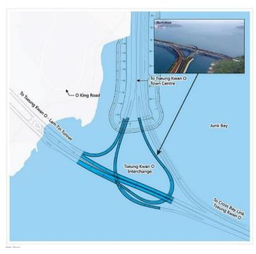
Project: NE/2017/01 Tseung Kwan O - Lam Tin Tunnel - Tseung Kwan O Interchange and Associated Works comprise construction of marine viaducts forming the TKO Interchange at Junk Bay
